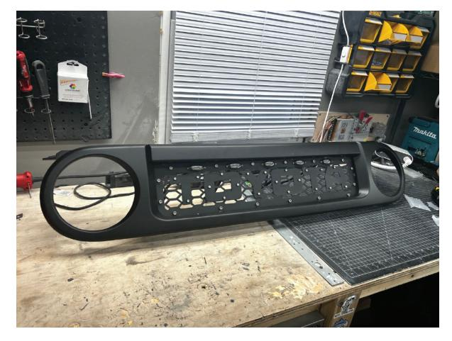
Accessory mounting hardware. On the outside of the grille insert there are 16 holes you can insert your accessory hardware to. Use your supplied bag of nuts and bolts to attach to the grille.
