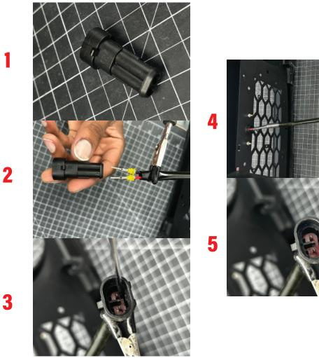
With the connector facing up, insert the red wire into (1) and the black wire into the (2) position
