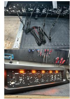
Grab your supplied harness, insert firmly into your raptor lights and wire into accessory switch or drl using a tap-a-fuse.
