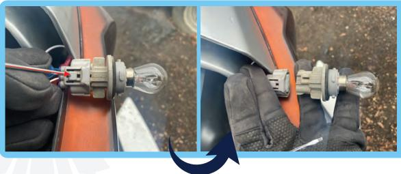
Take your Plug and Play Harness and insert in between your separated lightbulb socket and your OEM socket.
